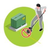
Don't dig near a transformer. Underground power lines can extend in any direction from it.
